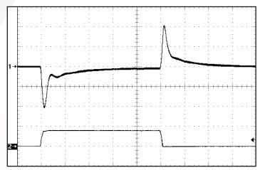
Figure 12: Output voltage response to step-change in load current 0%-50%-0% of Iout (max). Load cap:  $1\mu F$  ceramic cap and  $10\mu F$ ,  $100 \text{ m}\Omega$  ESR tantalum cap. Ch 1: Vout (200mV/div). Ch 2: Iout (104/div).
