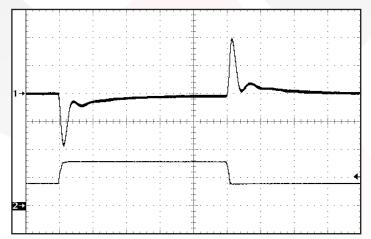
Figure 11: Output voltage response to step-change in load current 50%-100%-50% of Iout (max). Load cap:  $1\mu F$  ceramic cap and  $10\mu F$ ,  $100m\Omega$  ESR tantalum cap. Ch 1: Vout (200mV/div). Ch 2: Iout (10A/div).
